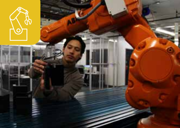
Sheridan engineering student at CAMDT conducts research on a collaborative project with industry exploring automated assembly in manufacturing, and making use of custom 3-D printed grippers and programming an industrial ABB robotic arm.
